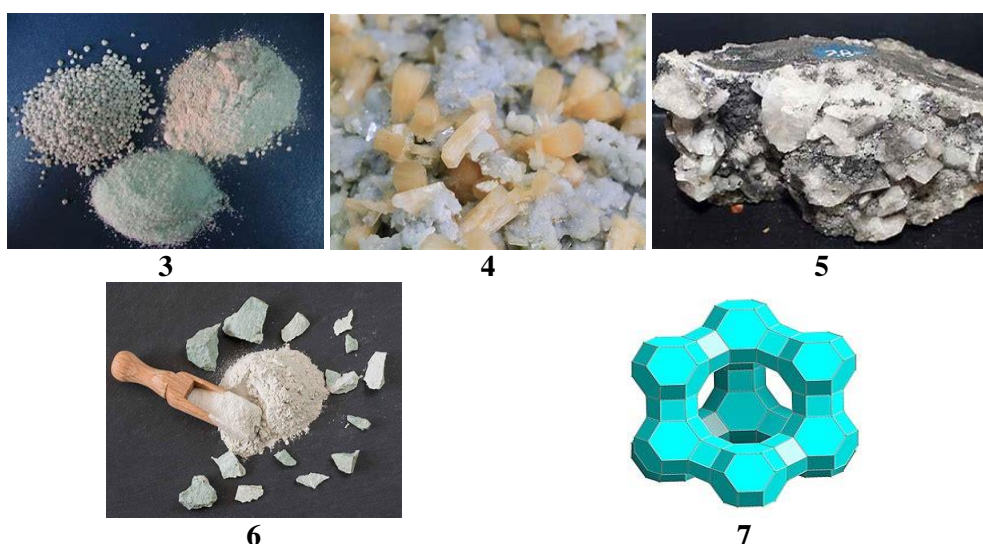
Figure 3, 4, 5, 6 and 7 Different forms and natural structures of zeolite, our examined zeolite is in the first and fourth group (figures 3 and 6)
